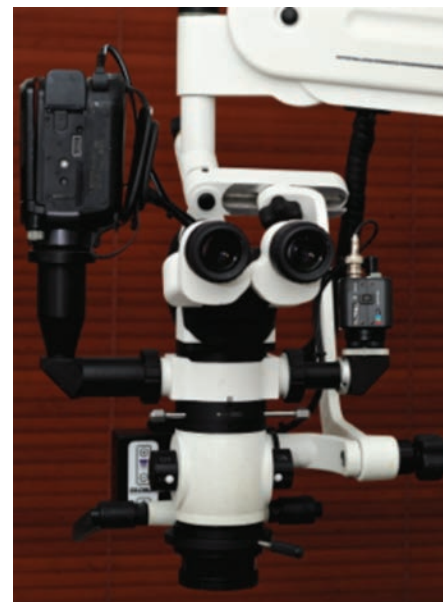
Figure 4: Global six-step dental operating microscope fitted with LED illumination
